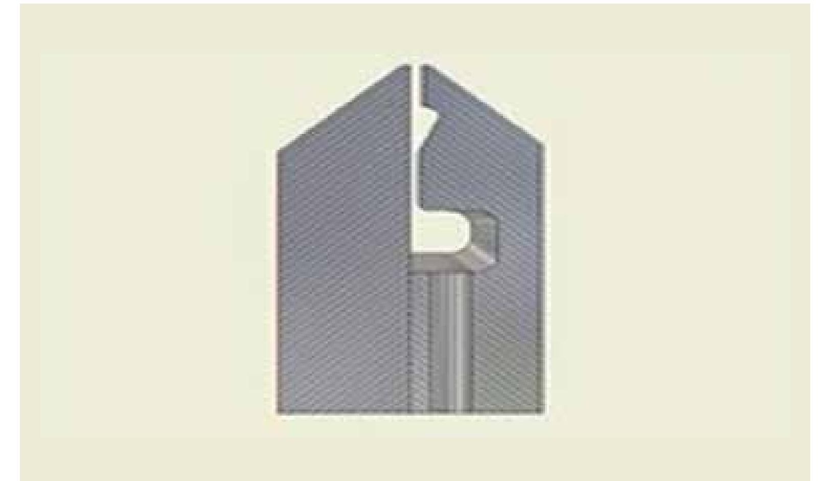
Slot Die section view displaying internal manifold
